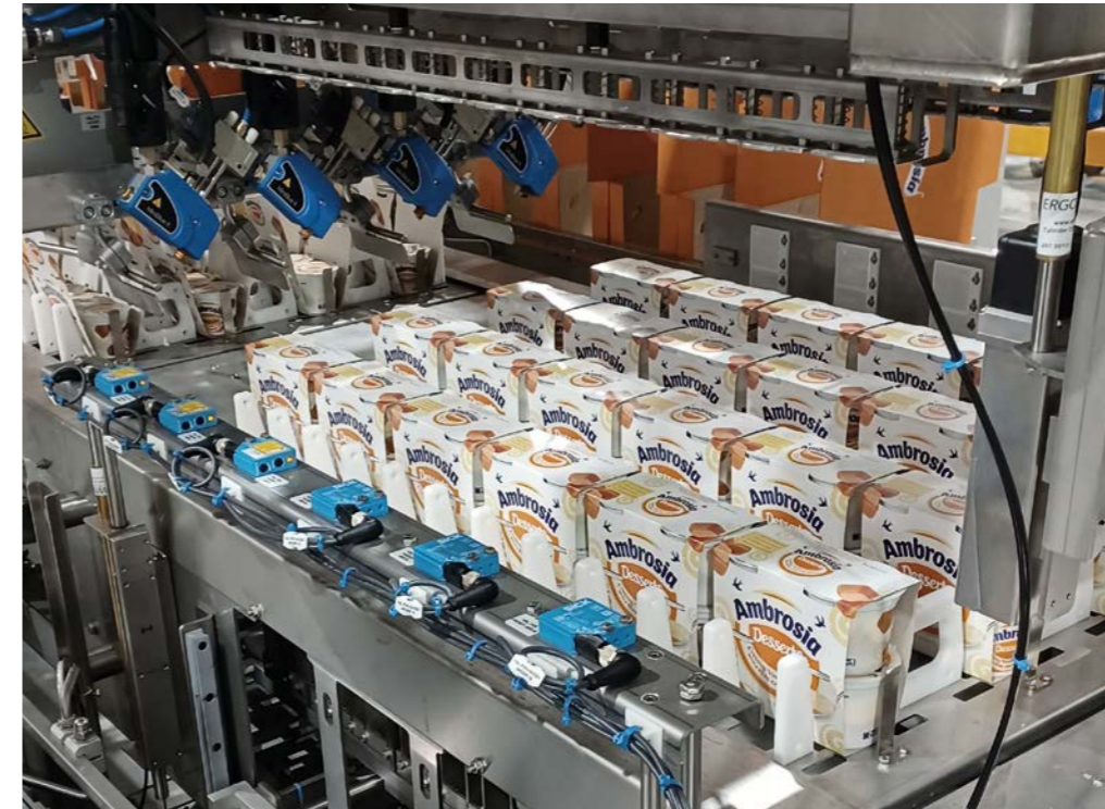
The SetLine sleeves up to 304 dessert cups per minute.
