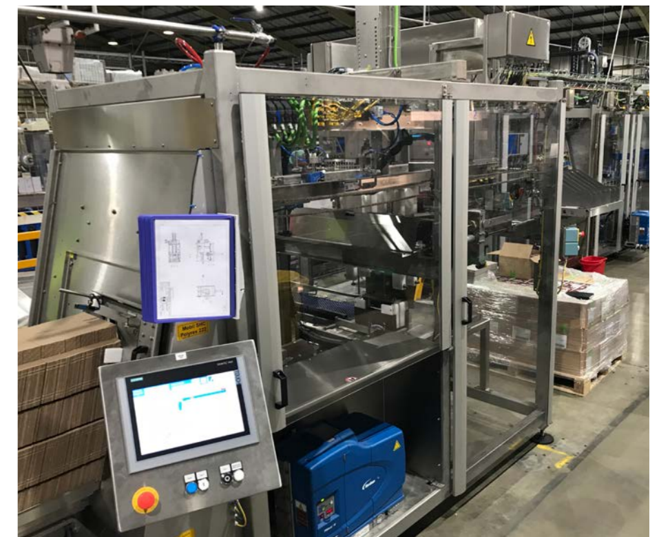
The tray erector, type MultiFormer, automatically forms the desired packs comprising sleeve and wraparound tray.
